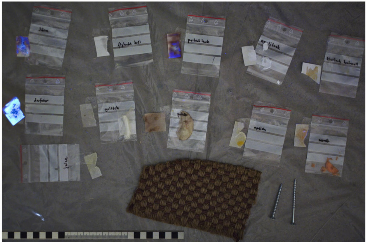
Fig: A forensic preparation of luminol where applied on samples of different household vegetables, chemicals and materials. The tests were performed merely to illustrate that false positive reactions are possible. All samples were prepared shortly before use. The amount of material on each filter paper varied. The quantity of luminol solution applied varied also considerably between the filter papers.
